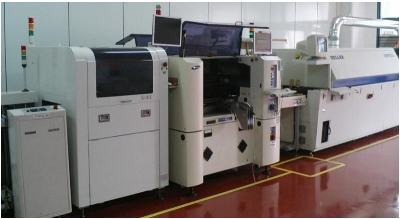
PaxDisk SMT Production Line with Reflow
