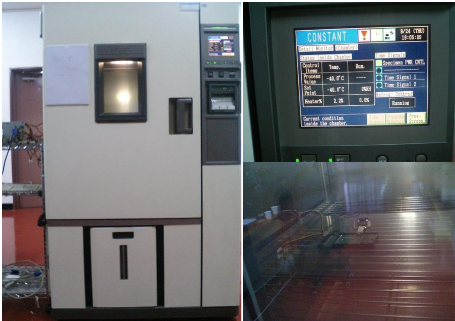
PaxDisk Temperature-Humidity Test Chamber
